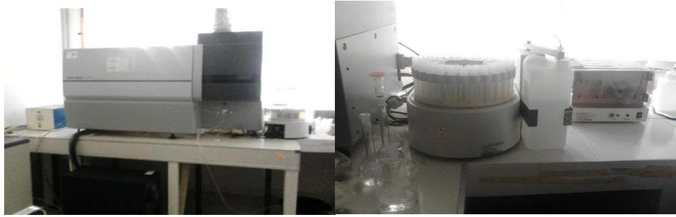
Gambar 21. Instrumen Alat Pengukur Cemar Logam Berat, ICPE ( Inductively Couple Plasma ) 9000 Shidmazu.
