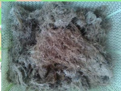
**Gambar 3.16** Serabut TKKS dari pabrik
