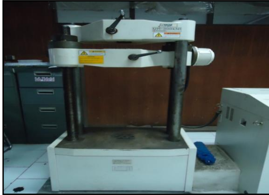
Gambar 1.6. Universal Testing Machine (UTM)
