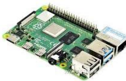
Gambar 2.10 Raspberry Pi 4B [165]
