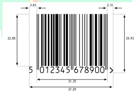
Gambar 1.3 1D Barcode Specification[9]
