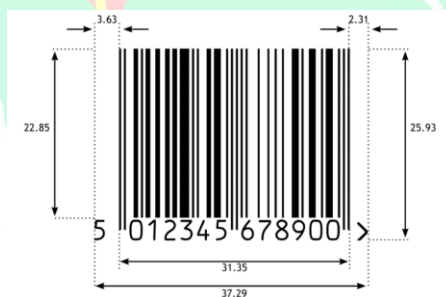
Gambar 1.3 1D Barcode Specification[9]
