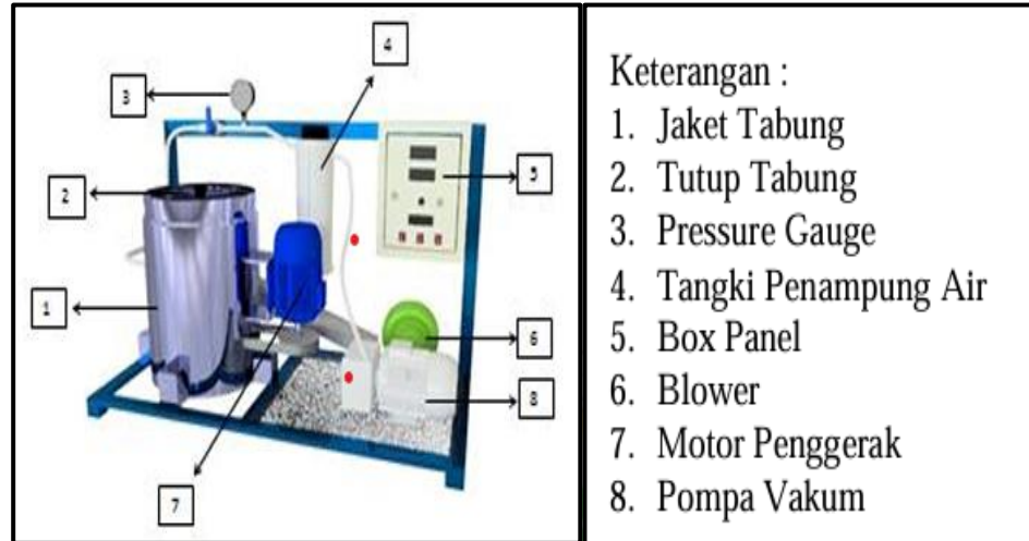
Gambar 2.5 Skema Alat Vacuum drying [52]
