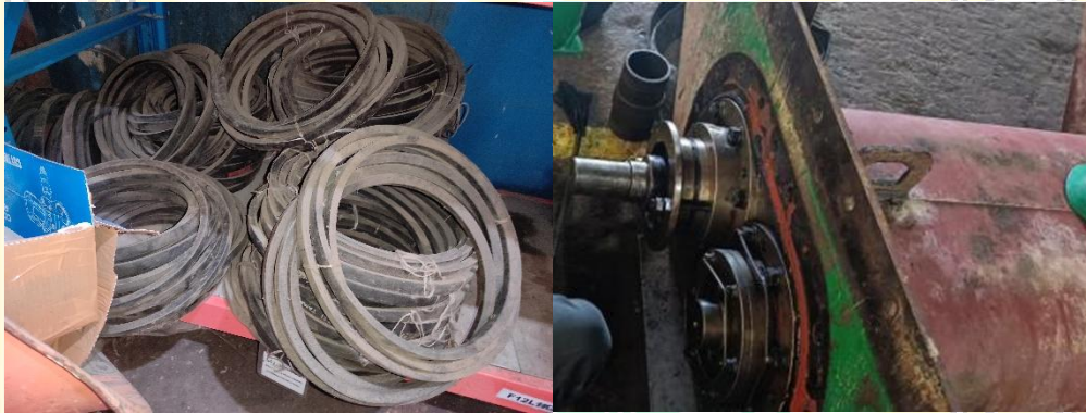
Figure 1.9 V-belt of The Vibrating Feeder
