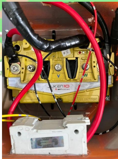
Gambar 4. 3 Controller Juken 10 72V
