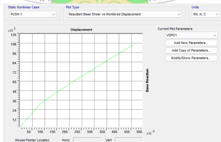
Gambar 4.54 Kurva Pushover – Y (Bangunan Retrofitting)
