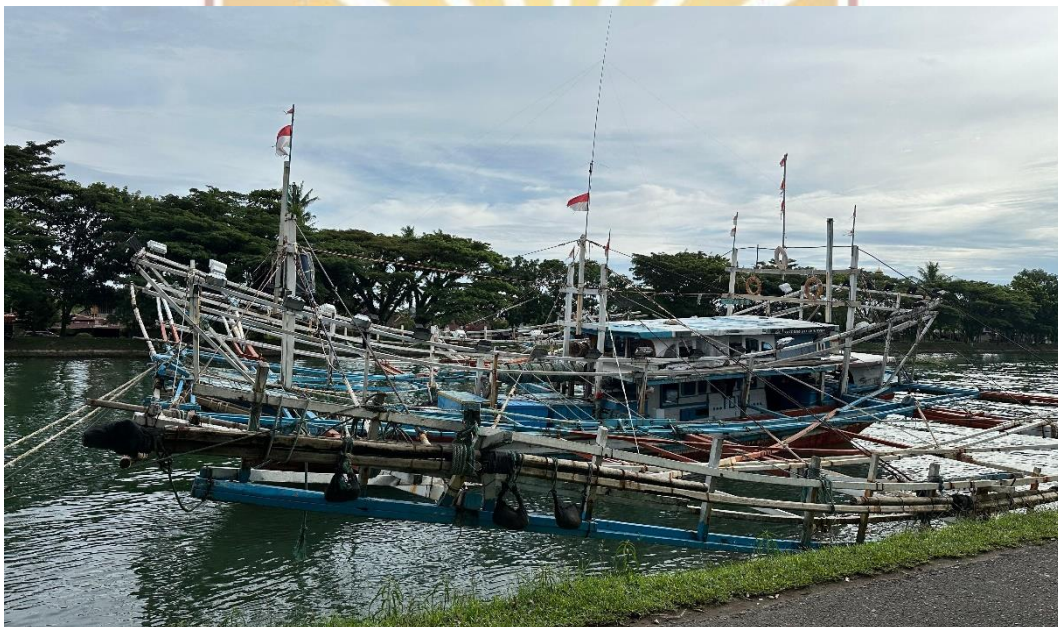
Figure 1.3 Fishing Vessels in the Study Area: Traditional lift net fishing vessel (kapal bagan) with outriggers and lights, representing vessels longer than 10 m that are currently impeded from accessing the floodway.
