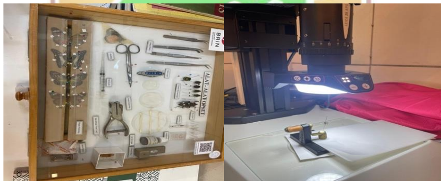
Figure 3. Offsets tools and camera lucida with software LA.S. 4.13,0 mounted on Leica Z6 APO Microscope.
