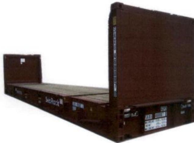
Gambar 2.11 *Flat rack container Collapsible type*
