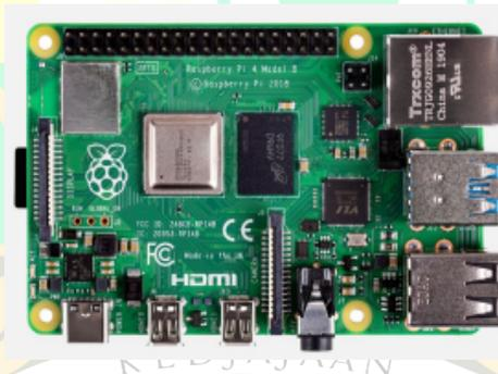
Gambar 2.4 *Raspberry Pi 4 Model B* [15]
