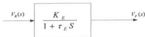
Gambar 2.4 Diagram Blok Exciter
