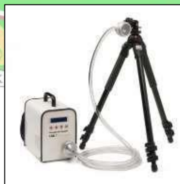
Gambar 3. 5 Low Volume Air Sampler (LVAS)
