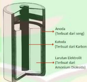
**Gambar 2. 1** Bagian-bagian baterai
