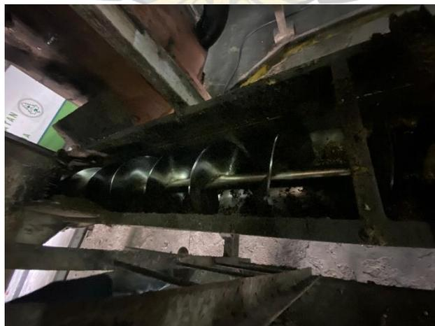
**Gambar 1.5** Mesin Conveyor Under Thresher
