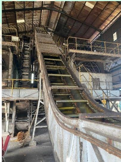
**Gambar 1.2** Mesin Discharge Fruit Scrapper
