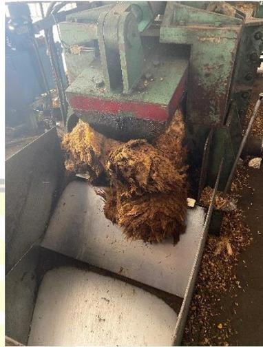
**Gambar 1.6** Mesin Bunch Press Pump
