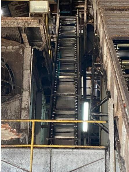
**Gambar 1.4** Mesin Re-thresher Scraper
