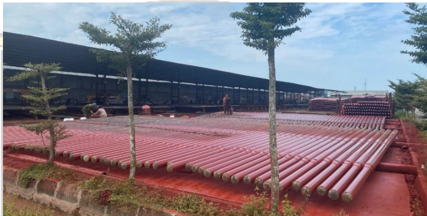
Gambar 1.2 Area Pengecatan Tiang Besi PT Tiga Pilar Sakato
