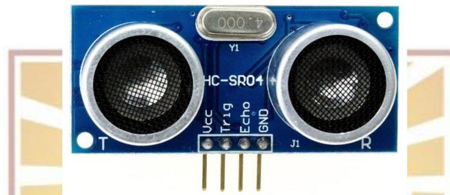
Gambar 12. Sensor Ultrasonik
