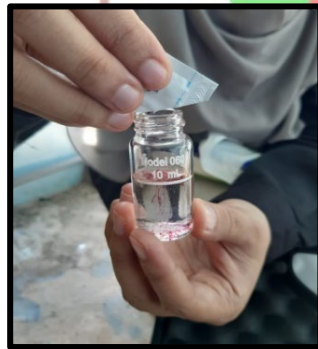
Gambar 3. 5. Penambahan Indikator Chlorine Free DPD
