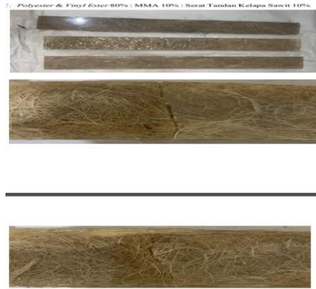
Gambar 3. 6 Polyester & Vinyl Ester (80%) , MMA (10%) , Serat Tandan Kelapa Sawit (10%)
