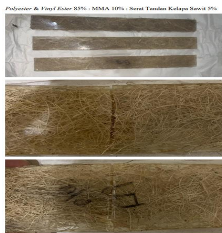
Gambar 3. 5 Polyester & Vinyl Ester (85%) , MMA (10%) , Serat Tandan Kelapa Sawit (5%)
