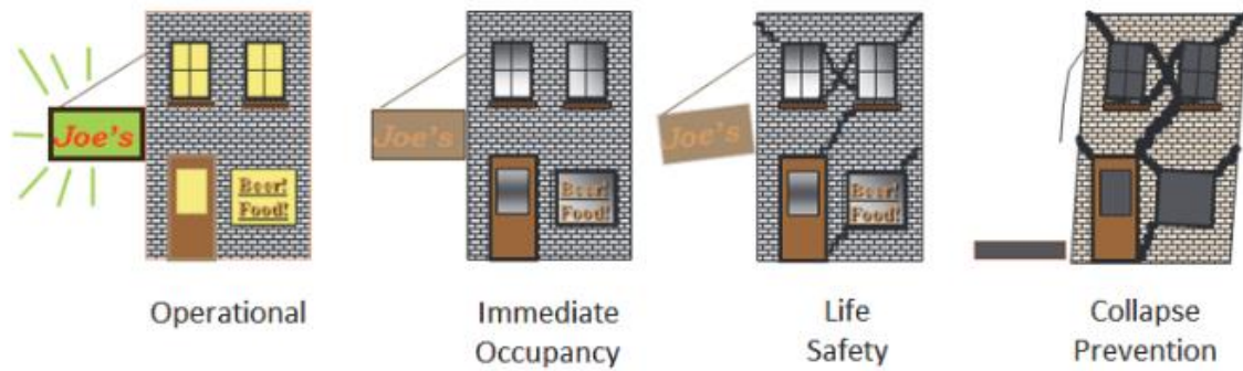
Gambar 1. 1 Standard structural performance levels berdasarkan Standard ASCE/SEI 41
