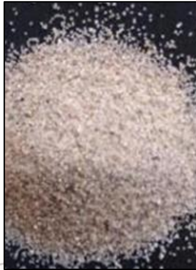
Gambar 3.19 Media Filter Pasir Kuarsa
