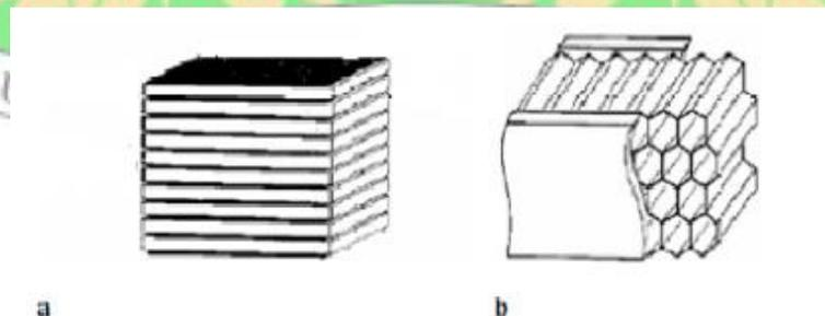
**Gambar 2. 6 a.** *Laminate* **b.** *Sandwich panels*
