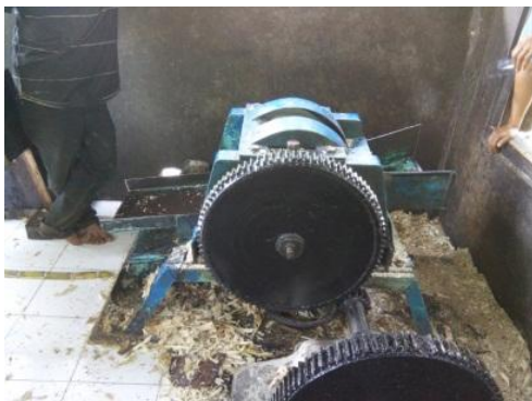
(a) Mesin kilang tipe 1 (3 unit)
