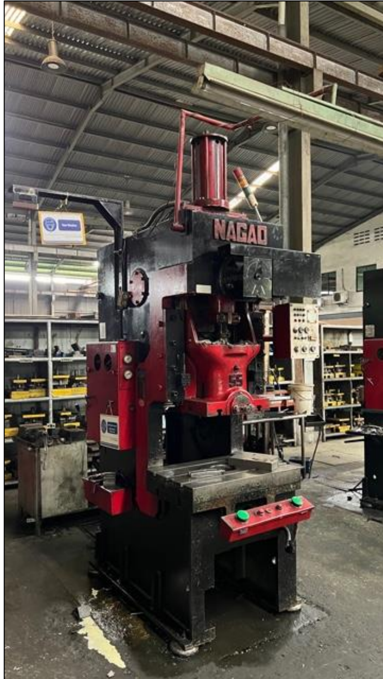
Figure 1.4 Hydraulic Press Machine Used for Producing Metal Work Products
