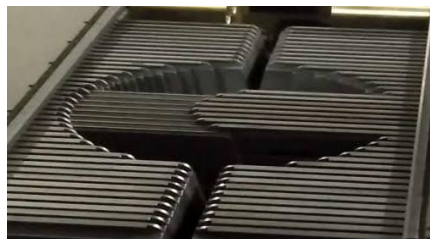
Gambar 2.11 Multi Leaf Collimator (MLC) (Sumber : Mayles, 2007)
