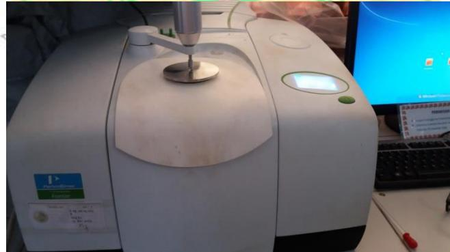
Gambar 28. Alat FTIR (PerkinElmer<sup>®</sup>)
