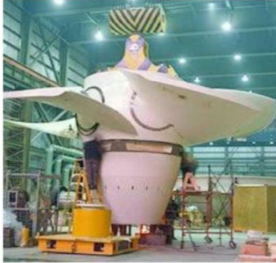
**Gambar 2.3** Turbin Propeller [7]
