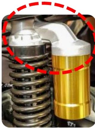
**Gambar 1. 1** Rear Cushion unit suspensi sepeda motor
