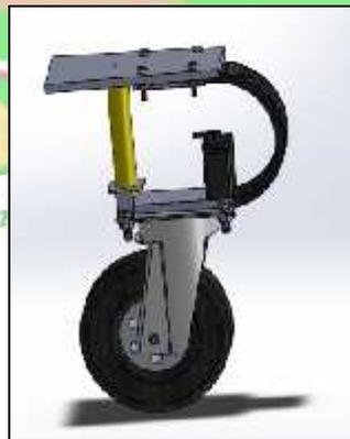
**Gambar 1. 2** *Nose Landing Gear*
