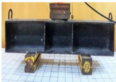
**Gambar 3.9 Spreader Beam**
