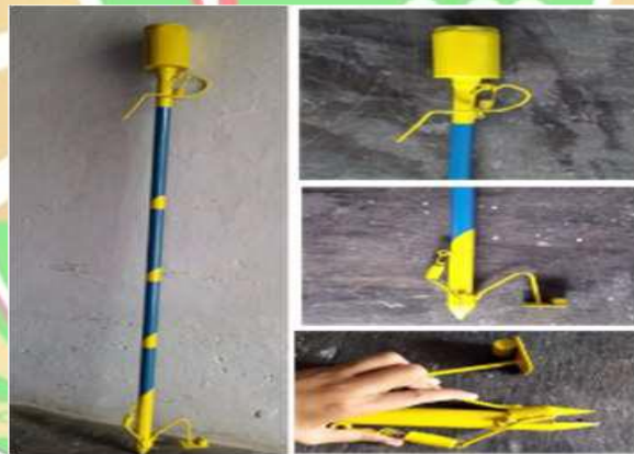
Gambar 7. Tugal Penanam Jagung Sistem Pegas Sumber : Sukmawati, (2021)
