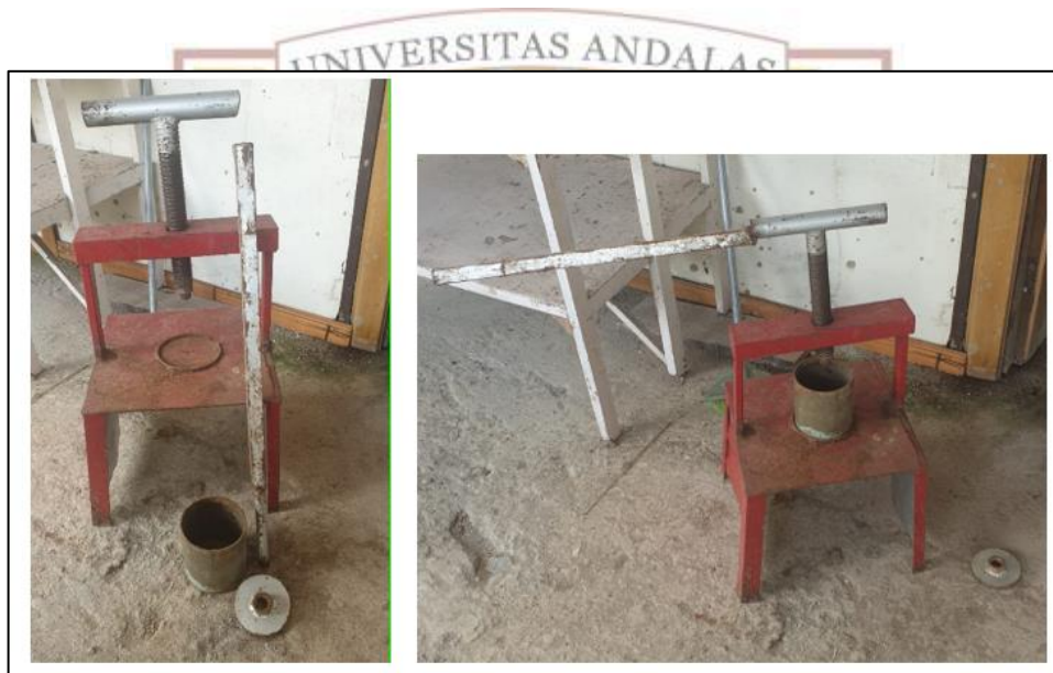
Figure 1.5. Molding machine used by MineFeeds.
